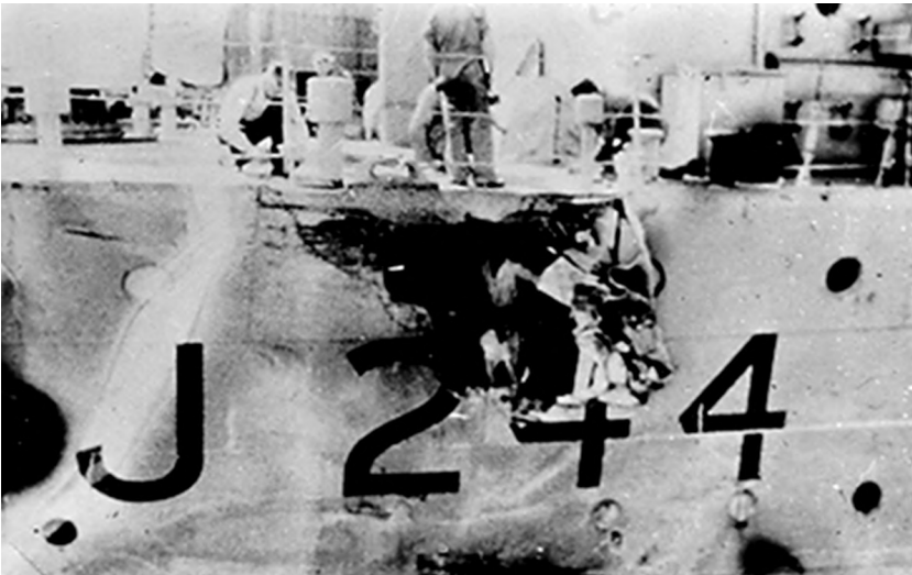
View of damage to the port side of Castlemaine
